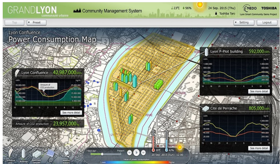
Monitoring screen of the district data collection and visualization platform (CMS) ©Toshiba
