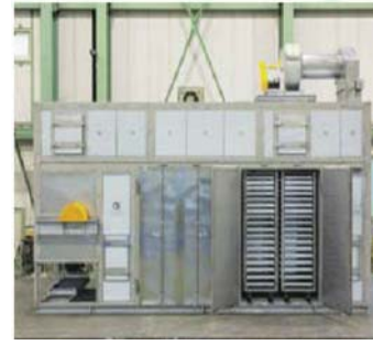
Tray Dryer (Box Dryer)
