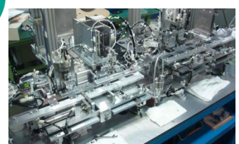
■ Iwaki Robotics Automation Project Automatic assembly machine for PV Connectors
